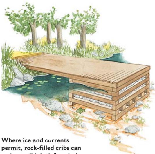
**Where ice and currents permit, rock-filled cribs can make a solid dock foundation.**
