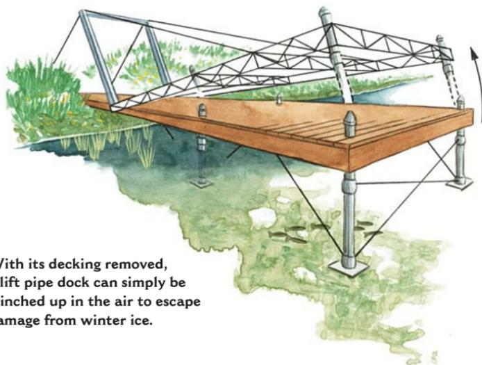
**With its decking removed, a lift pipe dock can simply be winched up in the air to escape damage from winter ice.**
