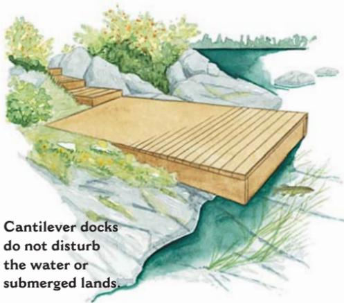
**Cantilever docks do not disturb the water or submerged lands.**
