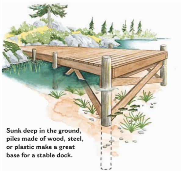
**Sunk deep in the ground, piles made of wood, steel, or plastic make a great base for a stable dock.**
