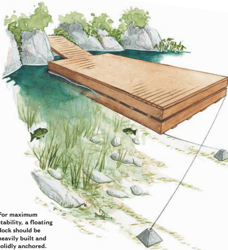
**For maximum stability, a floating dock should be heavily built and solidly anchored.**
